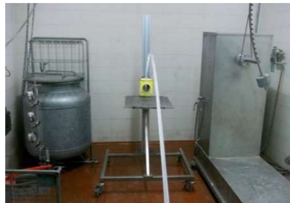
IP Test X5 (water)
