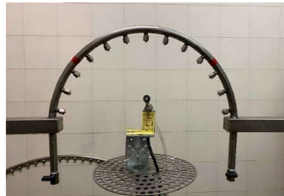
IP Test X4 (water)
