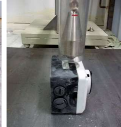
Impact test (cold)
